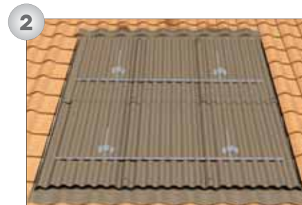
2) Flashings and collectors fixing carpentry installation.
