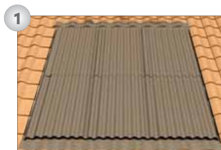
1) Carpentry removal and flashings placement.
