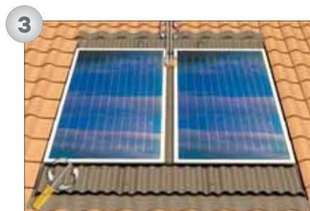
3) Collectors placing and fixing on the framework and fittings installation.
