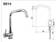
Special water saving perlator (Bubble flow, with Lime breaker, Flow rate: 8 I/min), Special cartridge with flow rate adjustment - With swivel spout, Length of outlet is 190 mm - Height of outlet is 255 mm, Measurements of Hot & Cold water flex hose connection are M10x1- 3/8"40 cm. Ideal operation pressure is 3 - 4 Bar
