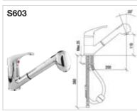
Special perlator with water saving, Special cartridge with heat and flow rate adjustment, With swivel spout, Removable hand shower head with 2 functions (Rain, Straight flow), Length of outlet is 225 mm - 125 cm helical hose (brass) - Height of outlet is 140 mm, Measurements of Hot & Cold water flex hose connection are M10x1-3/8"40 cm, Ideal working pressure is 3-4 bar
