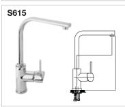
Special water saving perlator (Bubble flow, with Lime breaker, Flow rate: 8 I/min), Special cartridge with heat and flow rate adjustment- With swivel spout, Length of outlet 190 mm, Height of outlet 295 mm, Measurements of Hot & Cold water flex hose connection are M10x1- 3/8"40 cm, Ideal operation pressure is 3 - 4 Bar
