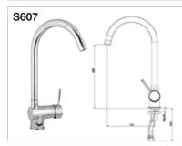
Special perlator with water saving (Bubble flow, with Lime breaker, Flow rate: 8 I/min), Special cartridge with heat and flow rate adjustment, With swivel spout, Length of outlet is 195 mm, Height of outlet 275 mm, Measurements of Hot & Cold water flex hose connection are M10x1- 3/8"40 cm, Ideal working pressure is 3-4 bar
