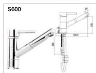
Special water saving perlator (Bubble flow, with Lime breaker, Flow rate: 8 I/min), Special cartridge with heat and flow rate adjustment- With swivel spout, Length of outlet 190 mm, Height of outlet 295 mm, Measurements of Hot & Cold water flex hose connection are M10x1- 3/8"40 cm, Ideal operation pressure is 3 - 4 Bar
