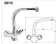
Special perlator with water saving (Bubble flow, with Lime breaker, Flow rate: 8 I/min), Special cartridge with heat and flow rate adjustment - With swivel spout, Length of outlet is 200 mm, Height of outlet 150 mm, Measurements of Hot & Cold water flex hose connection are M10x1-3/8"40 cm, Ideal working pressure is 3-4 bar
